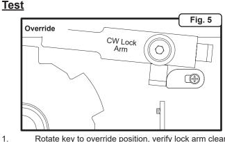
Rotate key to override position, verify lock arm clears cam shaft lobe and key is removable (Figure 5).
