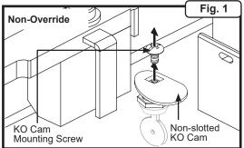
1. Rotate the key lock to the non-override position; then remove non-slotted key override (KO) cam (Figure 1).
