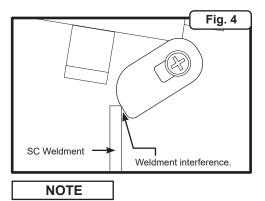
The self-centering (SC) support weldment may interfere with cam rotation. Modification of SC weldment to clear interference may be required (Figure 4).
