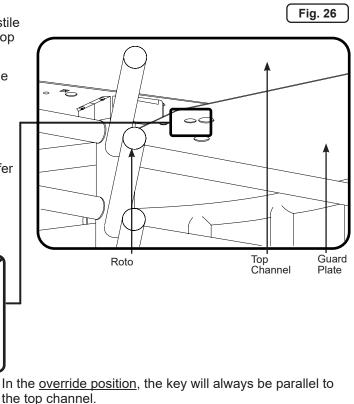
In the <u>non-override position</u>, the key will always be perpendicular to the top channel.
