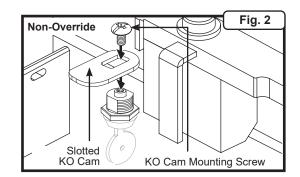
2. Install slotted KO cam. Do not fully tighten at this time (Figure 2).
