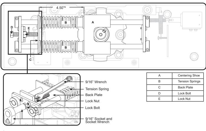
\* Dimension shown with Roto in the "home" position (no-load on tension springs).
