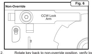
Rotate key back to non-override position, verify lock arm engages cam shaft lobe and key is removable (Figure 6).
