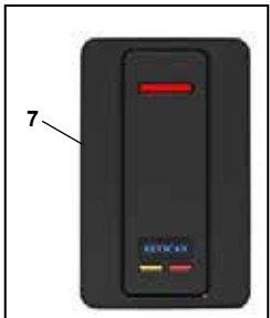
Fig. 5.1.3 Card reader example— by others
