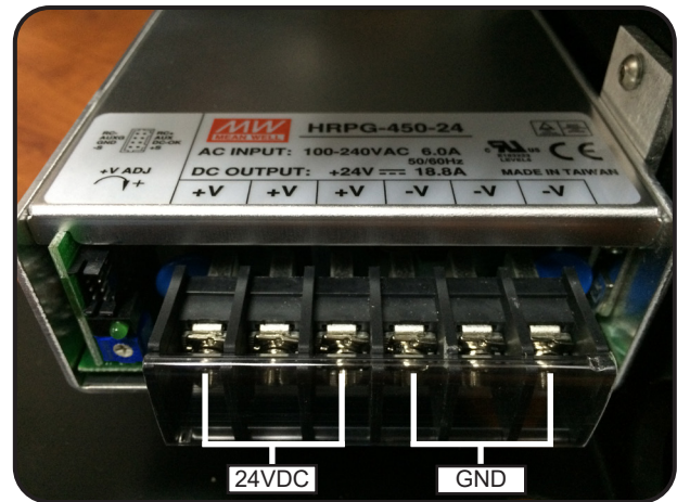
Fig. A4 Power Supply Output Terminal Block
