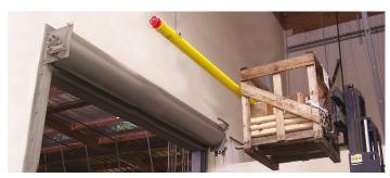
\*To avoid possible false alarms, the Watchman should not be installed, suspended or hung directly from a conveyor structure / frame work.
